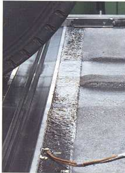
Edge sections butt-jointed at the centre of the wheel track. Thermocouple for temperature measurement.
