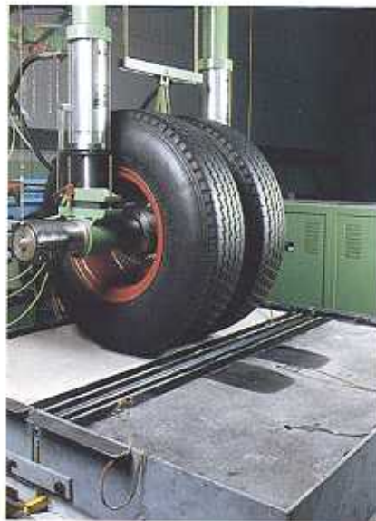
Wheel-load testing rig with test specimen.
